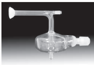
ES-3162-1118-26 Agilent Quartz Cyclonic Chamber for PC3
